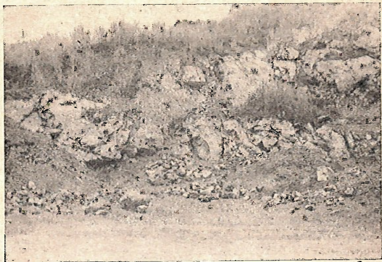
Fig. 1. An excavation to show the profile of Tacloban clay. The soil shallow and the andesite rocks are mined for road ballast.
