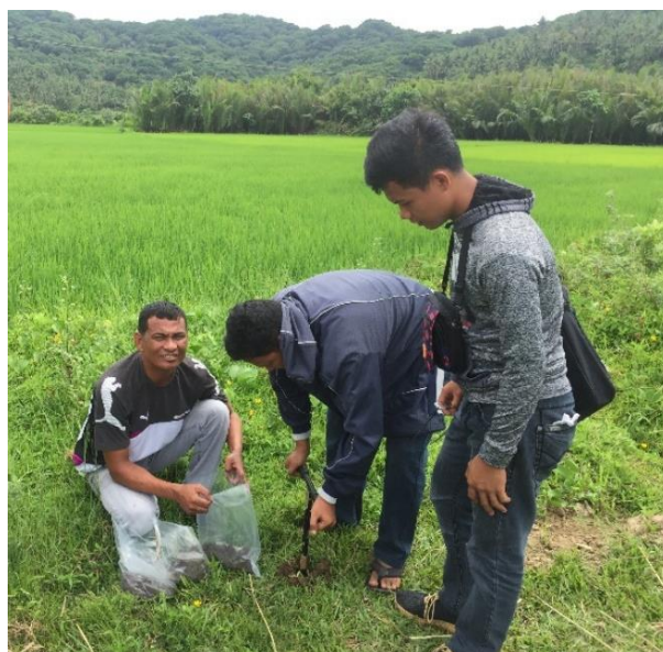
Figure 2.1 Auger Boring and Soil Sampling
