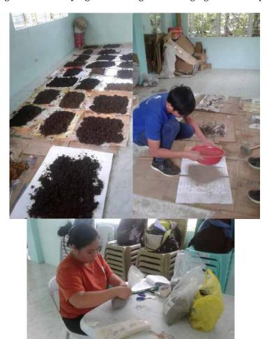
Figure 2.2 Air Drying, Pulverizing and Packaging of Soil Samples
