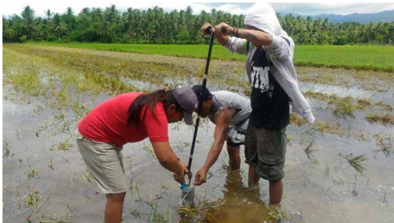
Figure 2.2 Auger Boring and Soil Sampling
