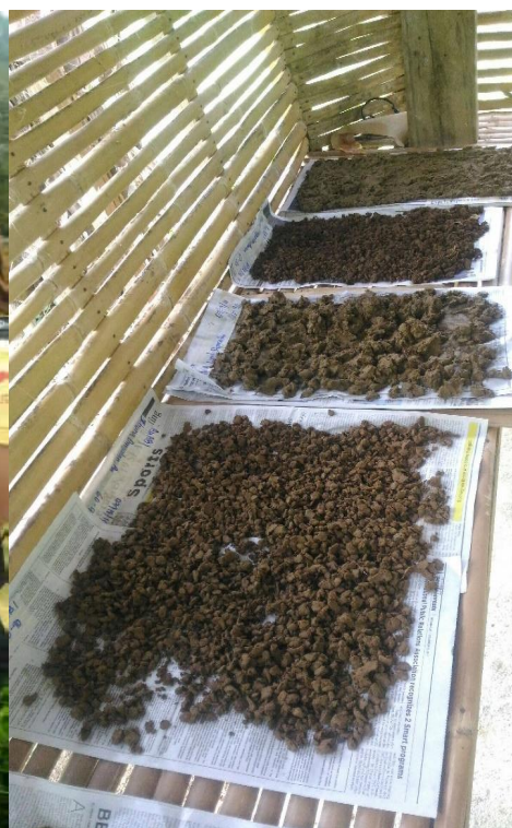
Figure 2.4 Air Drying of Soil Samples
