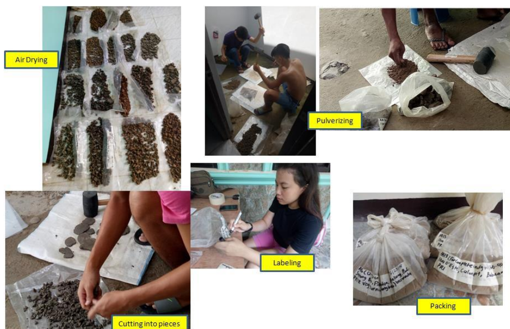
Figure 2.3 Air drying, pulverizing and packaging of soil samples
